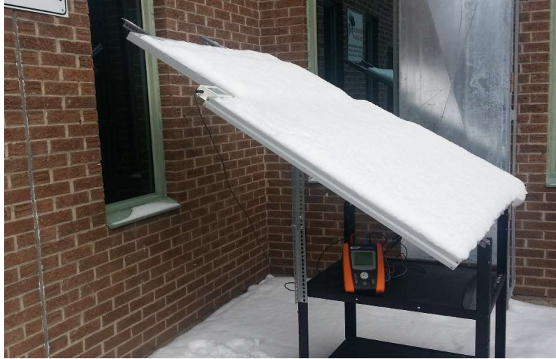
Figure 4.3 Experimental measurements of PV modules in cold months.
