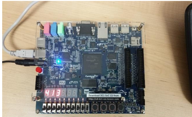
Figure 16. The code value and implement on DE1 Altera cyclone.
