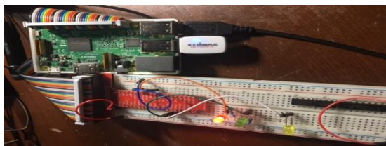
Figure 10. Led up to simulate the laser ablation.
