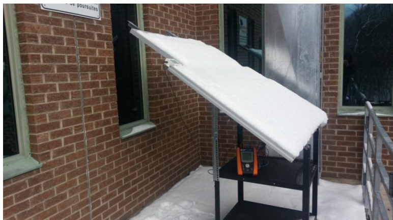
Figure 7. Experimental set-up for the snow-covered PV modules.
