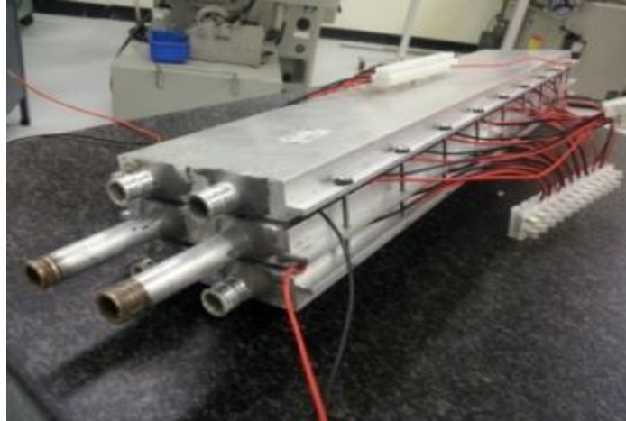
Figure 12: Thermoelectric generator composed of 40 modules and 3 heat exchangers for use with water
