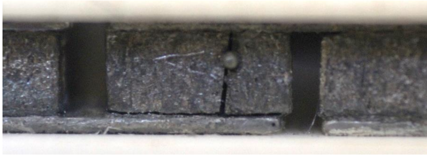
Figure 25: Picture of defects seen in the thermoelectric elements of module 1
