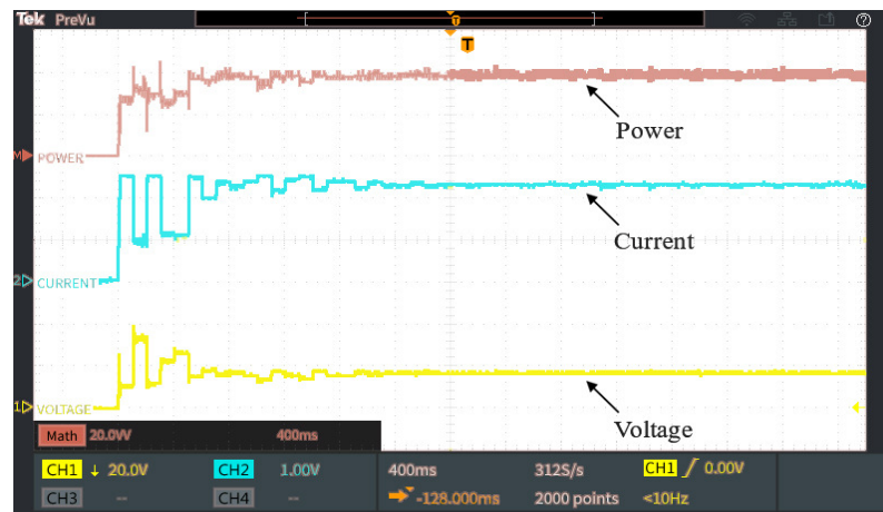
Figure 3.24: Generated power, voltage and current using traditional PSO algorithm for \omega , c_1 and c_2 equal to 0.3, 0.2 and 0.5, respectively.
