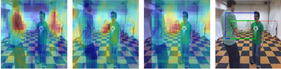
Figure 2.3.2 – Detection scores for two single person models (first and second image), the cumulative score (third image) and the final detection result (fourth image) [14].
