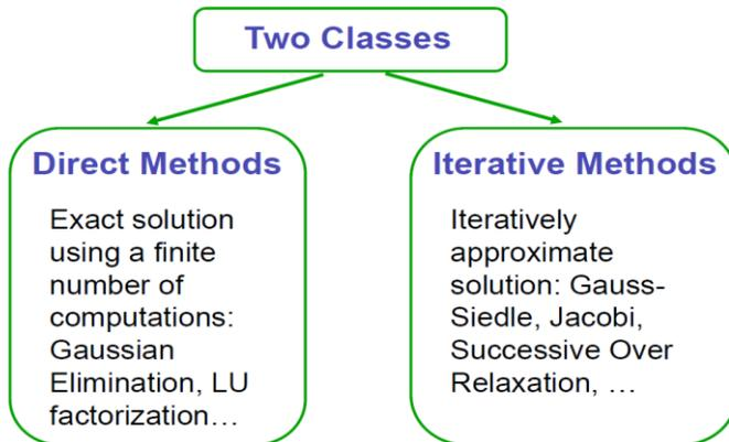
**Figure 12.** Numerical methods of solving linear algebraic equations.
