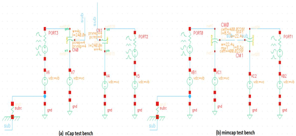
Figure 25. ncap and mimcap test bench characterization circuit.
