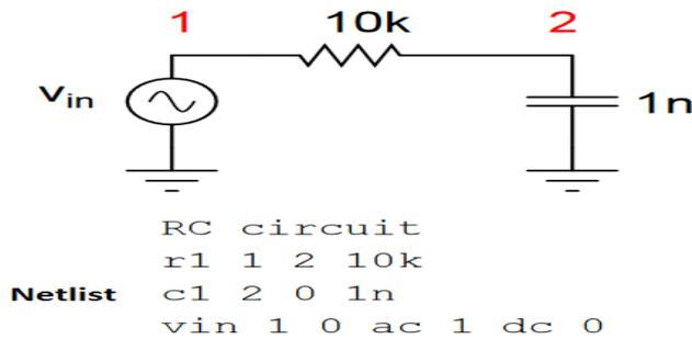
**Figure 7.** Example of an analog circuit and spice netlist.
