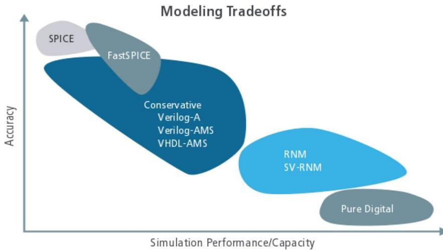
**Figure 15.** Simulation Performance of Analog and Digital Simulators [9].
