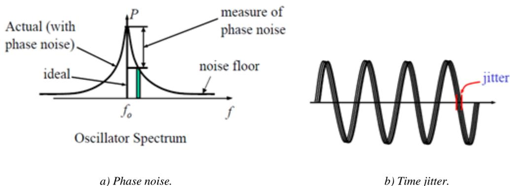
**Figure 40.** Phase noise and Time Jitter.
