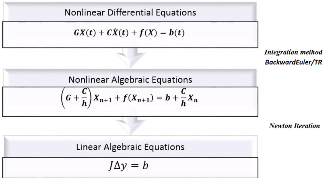
**Figure 11.** Numerical methods for transient analysis.
