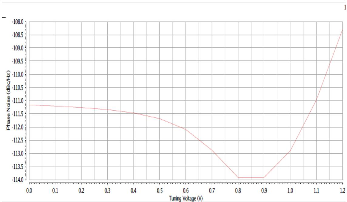
**Figure 36.** Phase Noise versus Tuning Voltage, tuning resistance = 100 Ohms.
