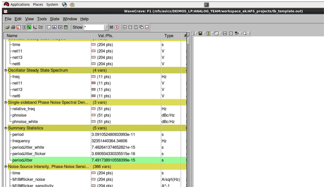
**Figure 41.** Fast spice analysis of Time Jitter of the physical model.
