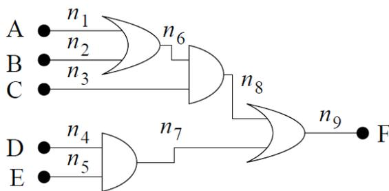
**Figure 3.** Combinational circuit.
