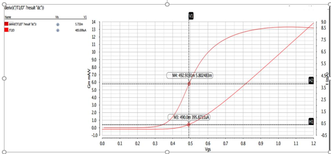
**Figure 23.** Transistor Characterization: gm and Ids versus Vgs.
