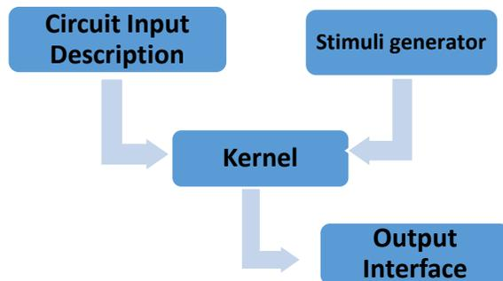
**Figure 2.** Structure of an analog simulators.
