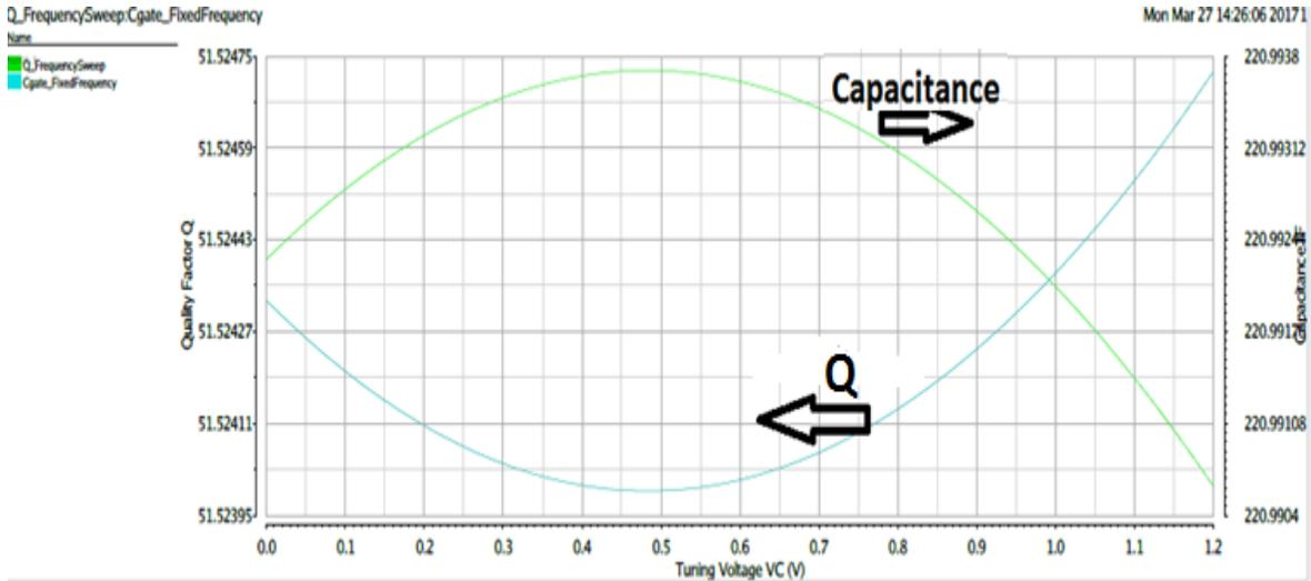
**Figure 28.** mimcap Characterization- biased at 1.2 V.
