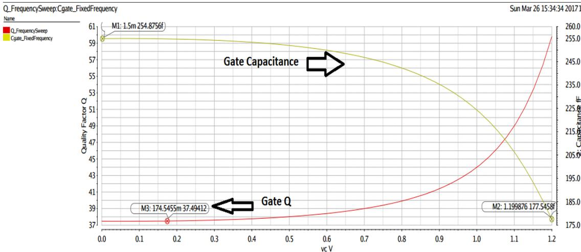
**Figure 27.** ncap Characterization: Gate biased at 1.2V
