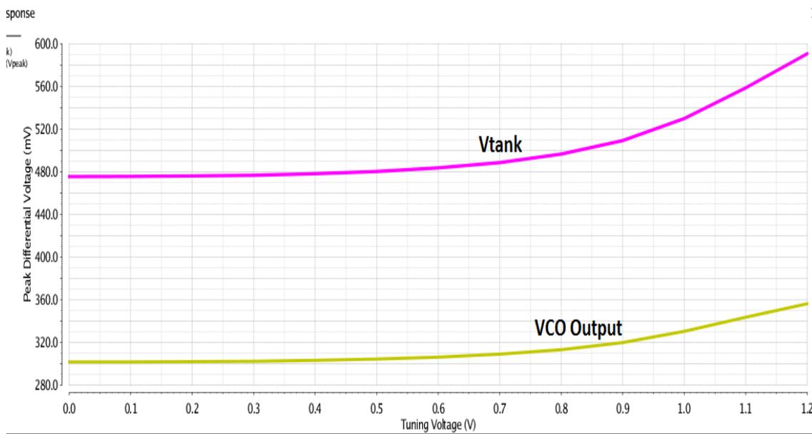
**Figure 32.** PSS Analysis: Tank and VCO output versus Tuning Voltage.
