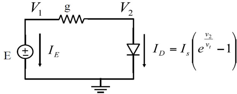
**Figure 9.** Example of a nonlinear circuit.
