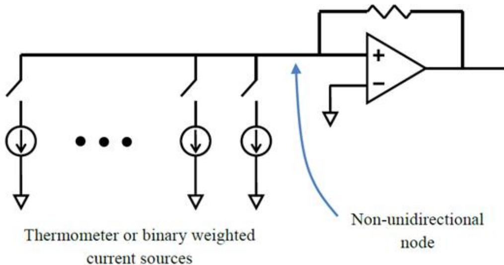
**Figure 18.** Summation node in analog circuits [17].
