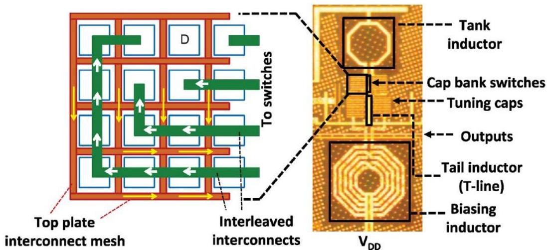
**Figure 46.** Typical VCO layout, adapted from [18].
