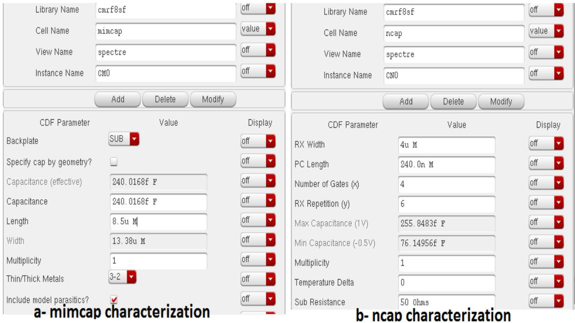
**Figure 26.** mimcap and ncap parameters.
