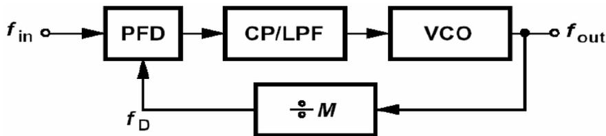
**Figure 47.** Analog PLL bloc diagram [36].
