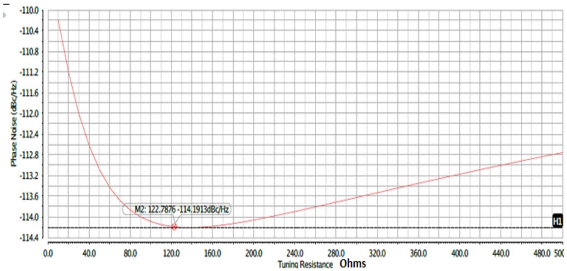
**Figure 37.** Phase Noise versus Tuning Resistance.
