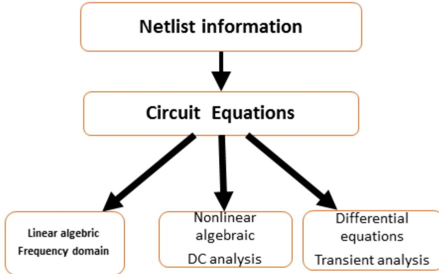
**Figure 10.** Three primary analysis methods [2].
