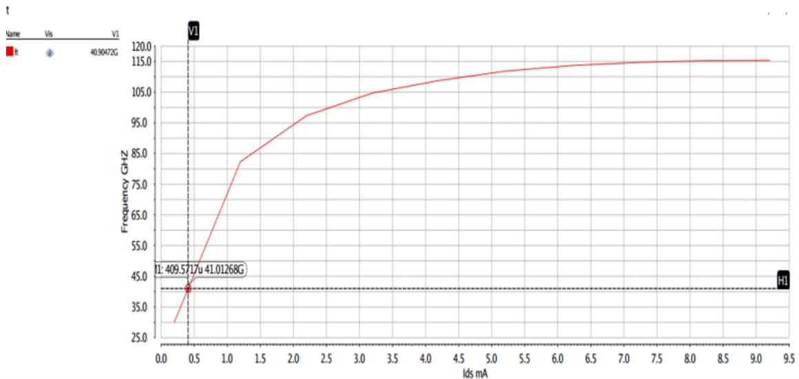
**Figure 24.** Transition frequency versus bias current.
