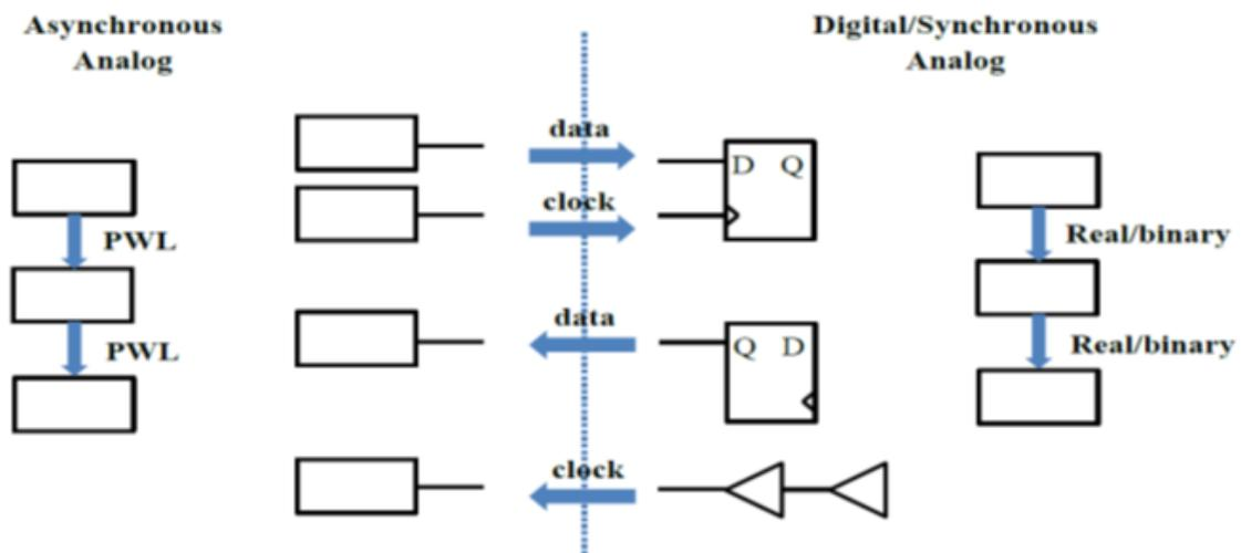
**Figure 20.** Communication between Analog/Digital components.
