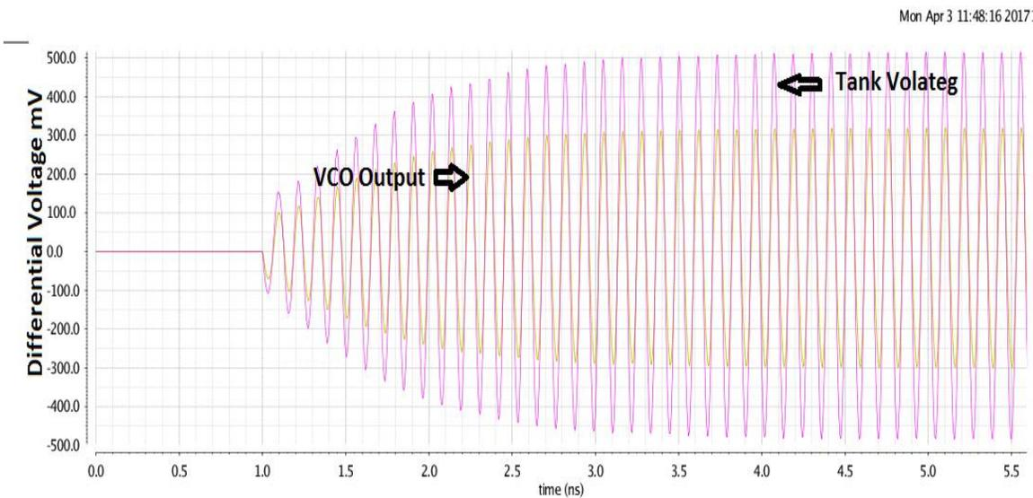
Figure 30. Transient Analysis: Tank and Output voltage.
