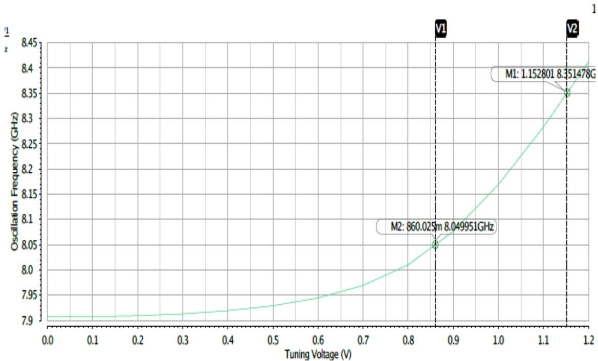
**Figure 31.** Frequency Range versus Tuning Voltage.
