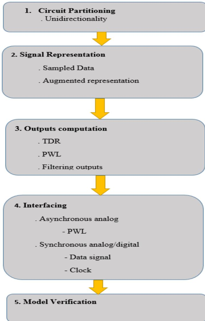
**Figure 17.** Proposed Framework for Mixed-Signal Verification.
