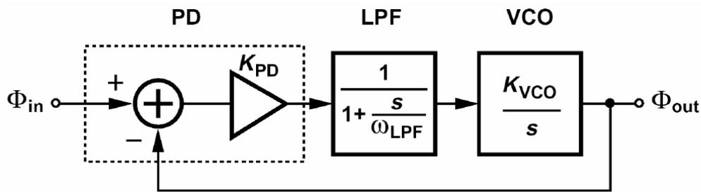
**Figure 48.** Contribution of each bloc to PLL phase noise [36].
