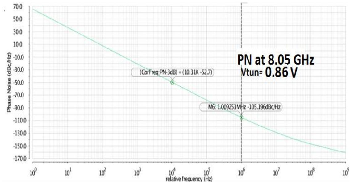
**Figure 33.** Initial design: Phase noise at 1 MHz offset
