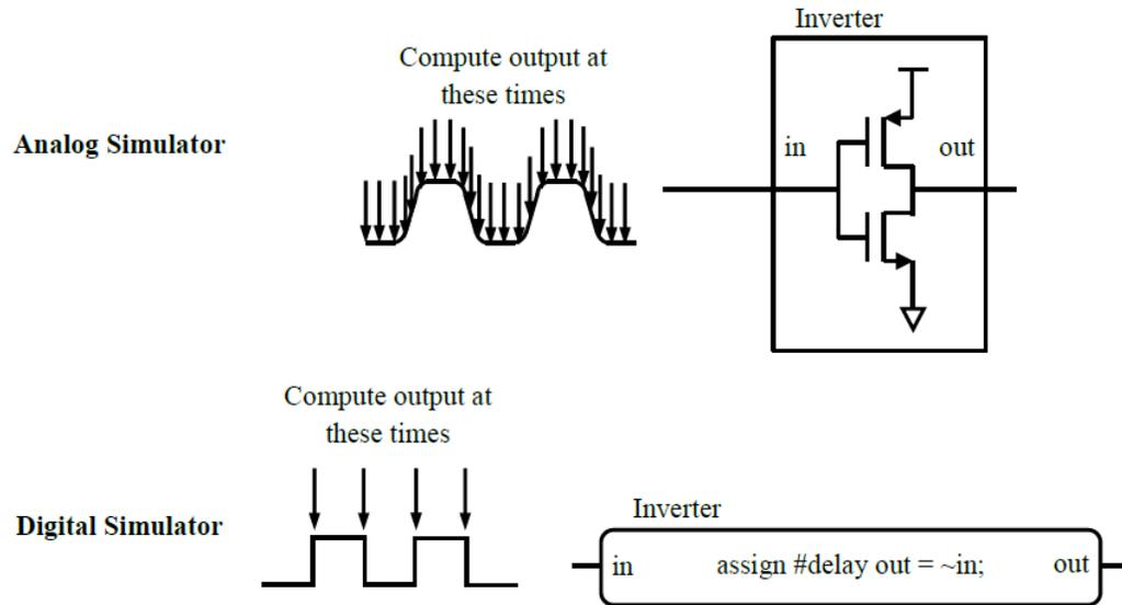
**Figure 13.** Simulation time in Analog and Digital Simulators.
