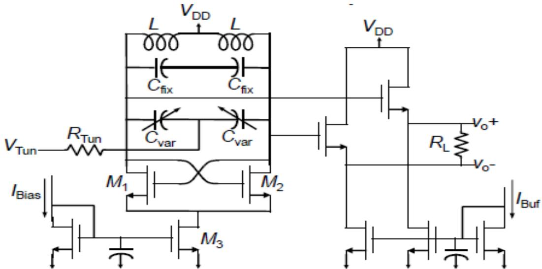
**Figure 22.** –Gm CMOS differential oscillator.
