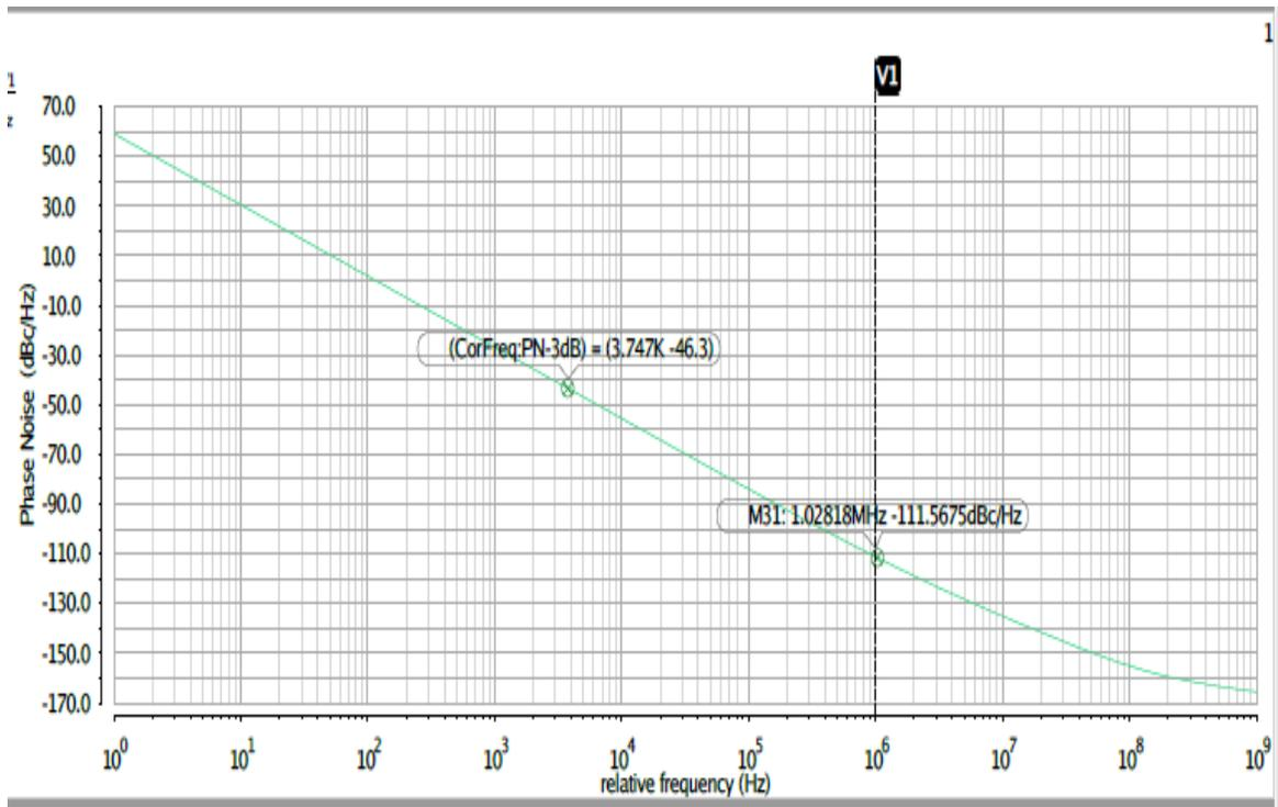
**Figure 35.** Phase Noise of the final design at offset 1Mhz.
