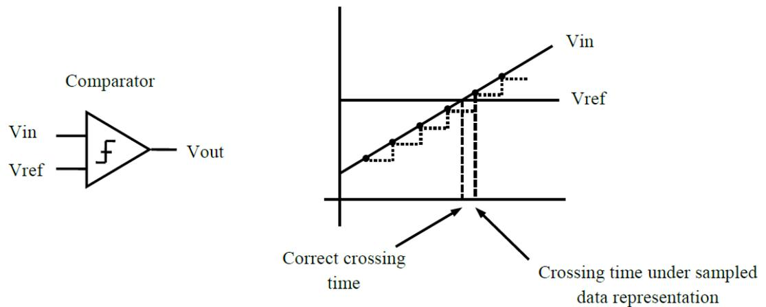
**Figure 19.** Sampled Data Representation of an analog comparator.
