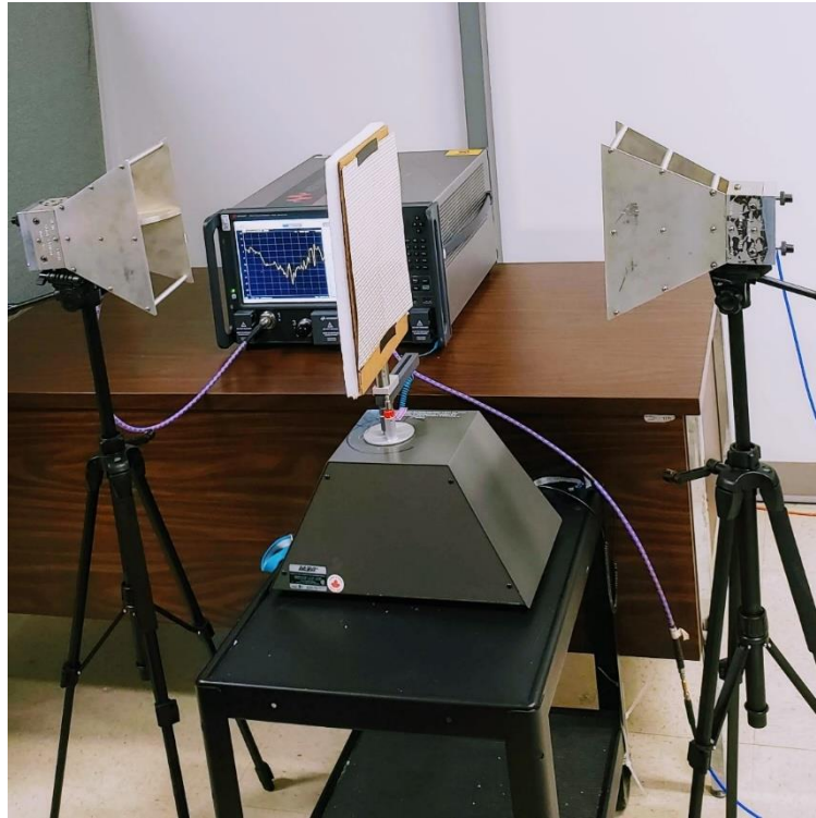
Figure 5.5 Measurement setup to measure the transmission coefficient of the FSS.
