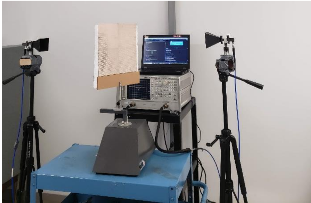
Figure 4.14 Measurement setup to measure the transmission coefficient of the MS.
