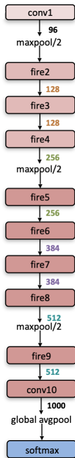
FIGURE 2.13 – SqueezeNet V2 architecture [11]
