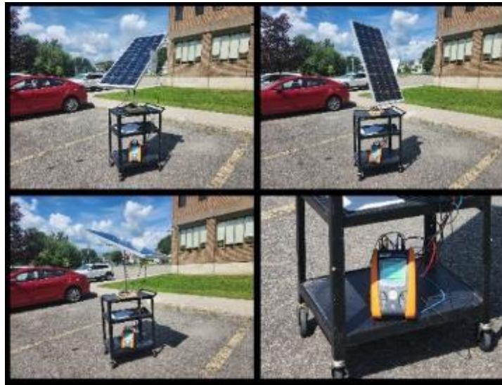
Figure 3.15. Experimental setup including ET-M53695 moving PV module, I-V 400 PV analyzer, irradiance and temperature sensors.
