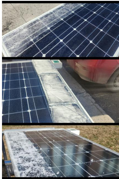
Figure 5.9. Experimental tests by simulating of various kind of ice from top: glaze, mixed and rime.
